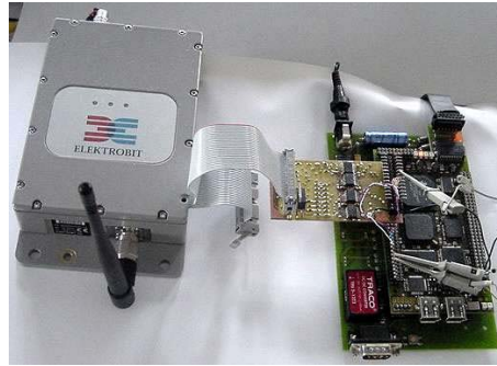
Figure 2.23. Medium Access platform. RF modem and DSP board are connected through a small custom-made adapter board (level shifters for voltage level conversion).
